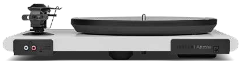
ABOVE: Stereo RCA sockets are mounted under the left of the plinth while the 5V 'wall wart' PSU plugs in on the right. Note the minuscule 'Passive/Active' switch adjacent to the RCAs that enables the in-built phono stage [see boxout, p65]
